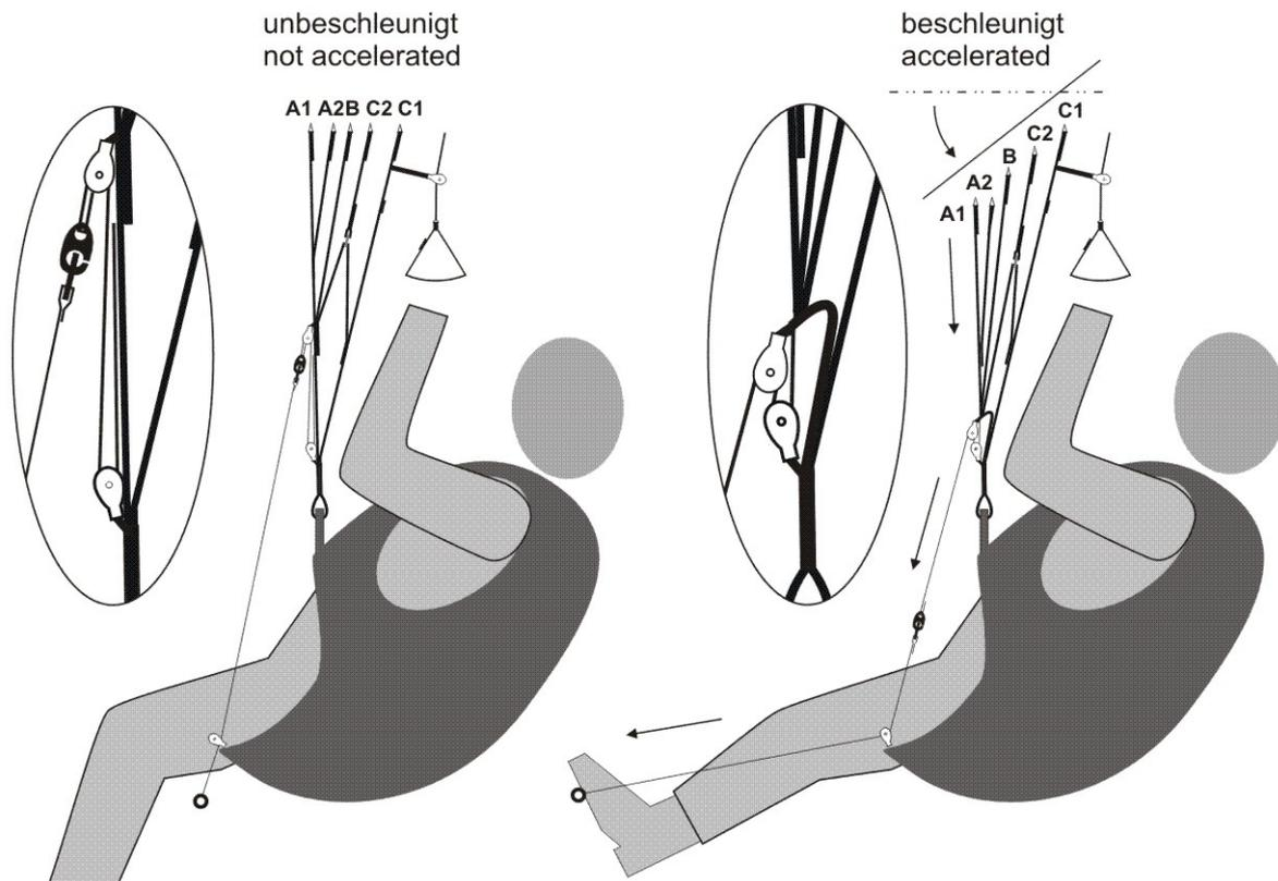
**Figure 2: How the Speed system works**
